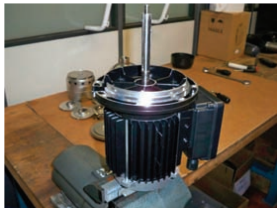
23. Put motor up side down and lock the shaft with a bench vice.
