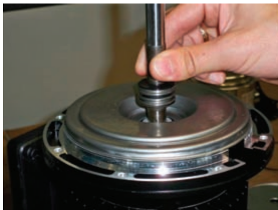
11. Insert the specific tool /pipe having very fine wall) between the rubber of the mechanical seal and the shaft. Pull the tool holding the mechanical seal upwards to the end of the shaft.
