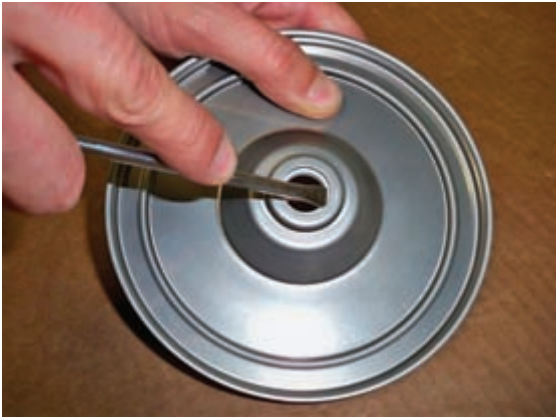
13. Remove the static portion of the mechanical seal from the seal plate.
