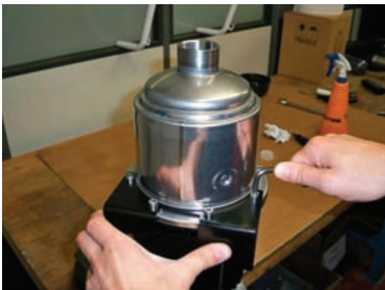
34. Secure the pump casing to the motor by tightening the pre-loading screws.
