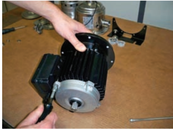
14. Unscrew and then remove the tie bolts.
