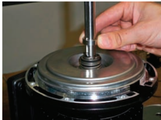
10. Remove the mechanical seal locking disk, split rings and washer.
