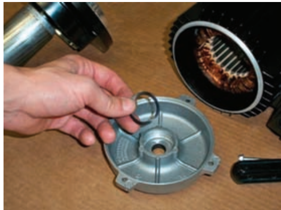
16. Remove the motor cover and the compensation ring.
