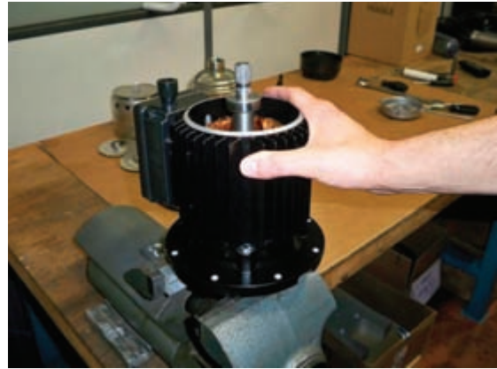
19. Couple the stator 19. Insert the rotor into motor flange. with motor flange.
