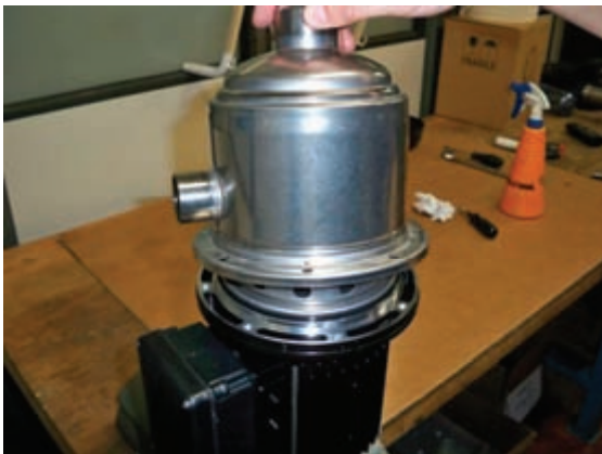
32. Lubricate the O-ring with alcohol and then position the pump casing.
