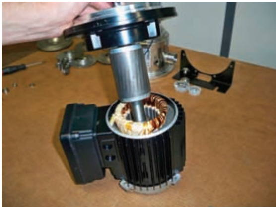
15. Pull out together the rotor and motor flange.
