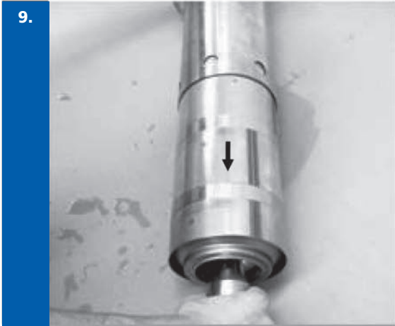
9. Pull out hydraulic group (stages+ pump shaft + coupling).
