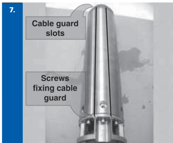
Align holes and slots to fix cable guard between discharge head and motor adapter.
