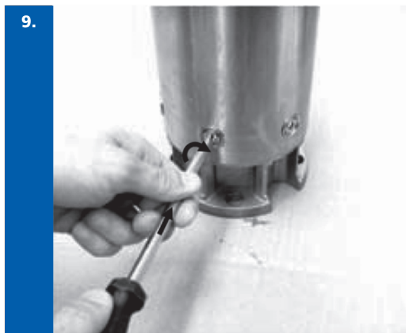
Screw in M8 screws fastening locking inserts.
