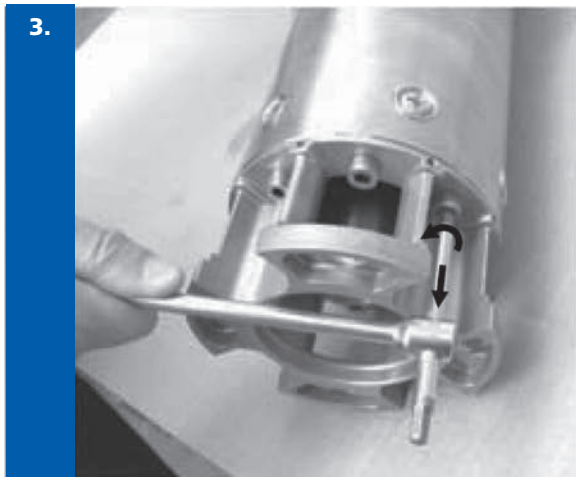
Screw out clamping screws diagonally little by little until they are completely unloosed.
