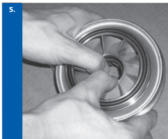
Pull out upper bearing bush from upper bowl.
