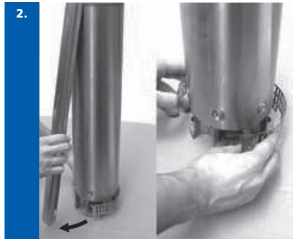
Remove cable guard and suction strainer.
