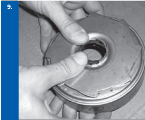
Remove secondary bearing bush from diffuser (radial flow stage diffuser).
