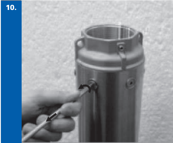
10. Repeat operations 5-6-7 to remove discharge head.
