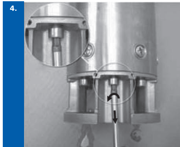
Keep some space between motor adaptor and top of the screws.
