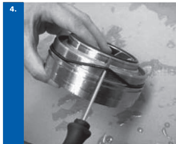
Remove upper bowl sealing o-ring.
