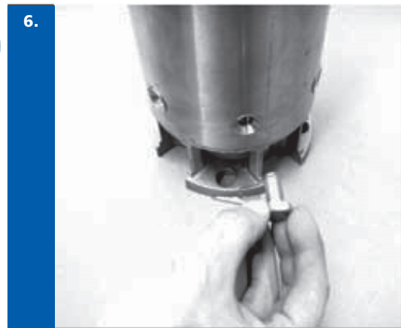
Use a M10 screw to remove locking inserts.
