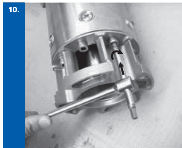
Screw in clamping screws diagonally little by little until motor adapter is perfectly coupled to outer case.
