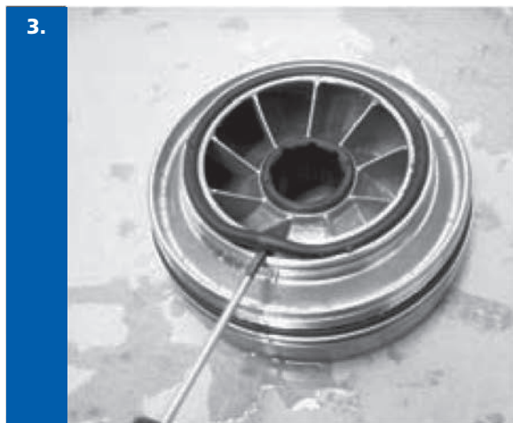
Remove valve disk sealing o-ring.
