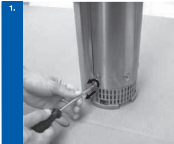
Screw out the two M4 screws fastening cable guard.
