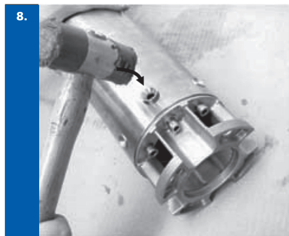
Insert locking inserts by hand or using a plastic mallet.
