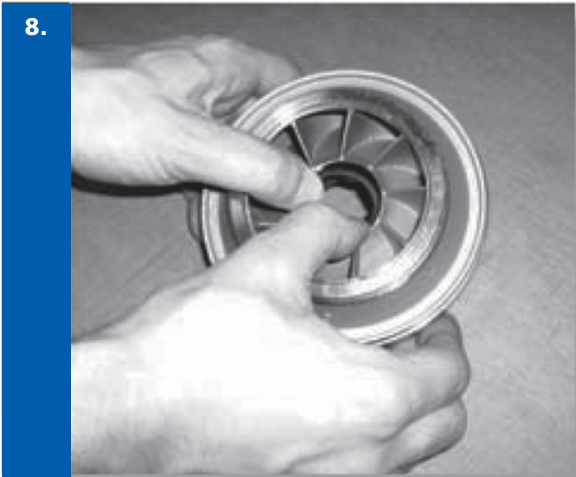
Remove secondary bearing bush from diffuser (mixed flow stage diffuser).
